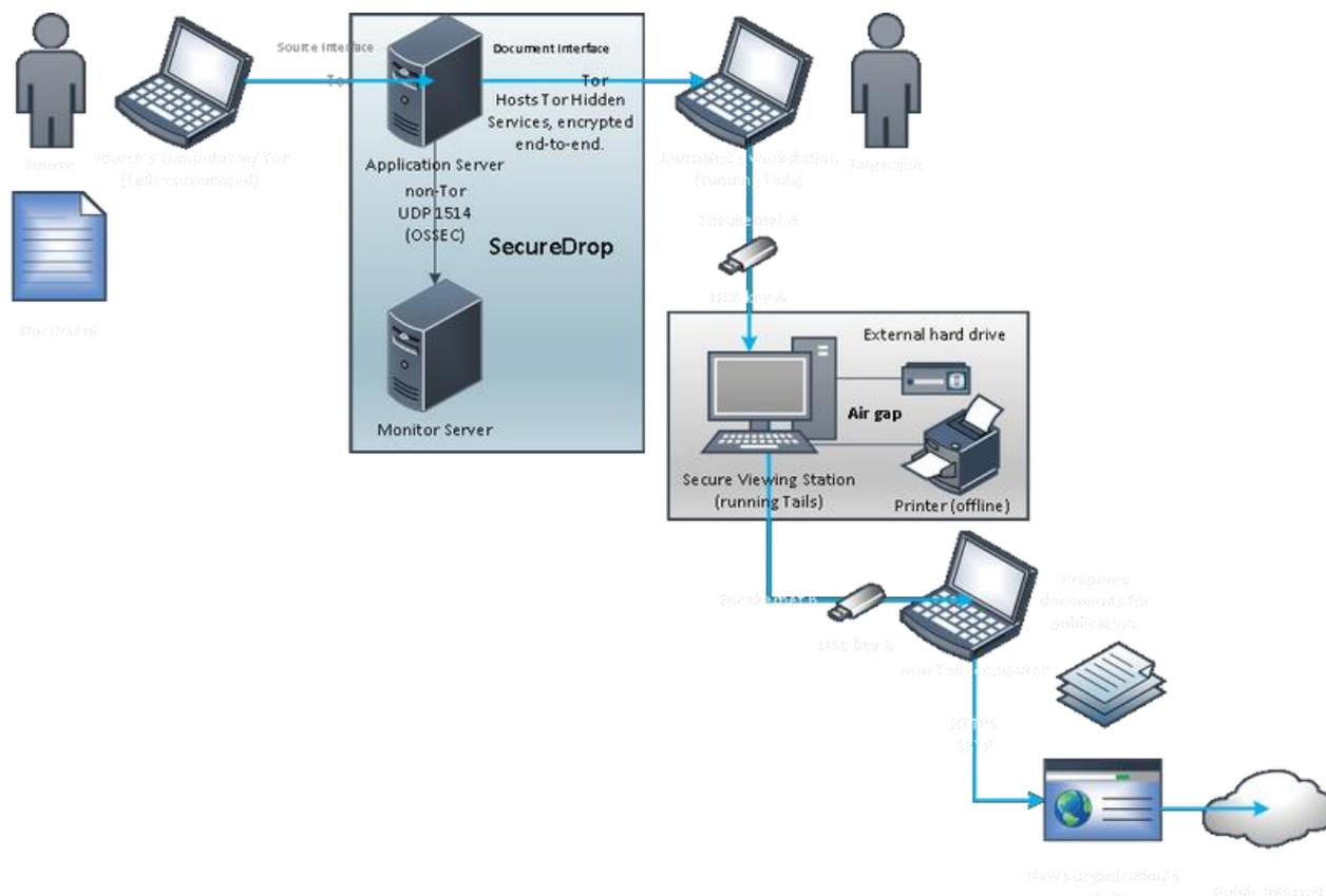
Figure 2: SecureDrop architecture
